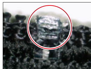
Coil zipper (P-TOP) damage example
